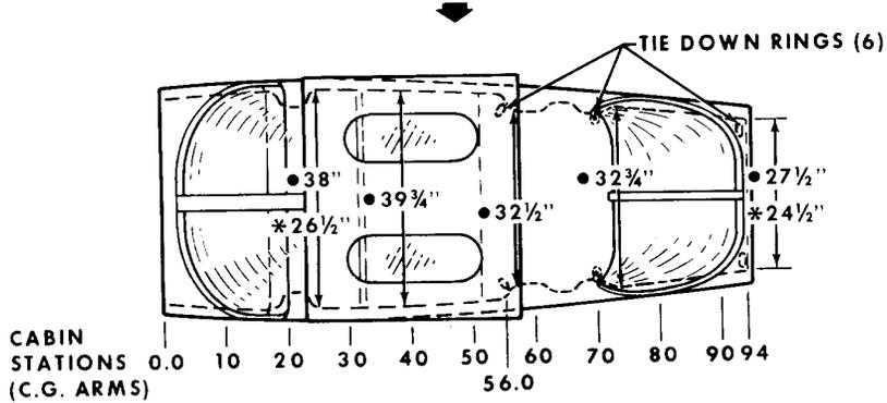
Figure 6-5. Internal Cabin Dimensions
