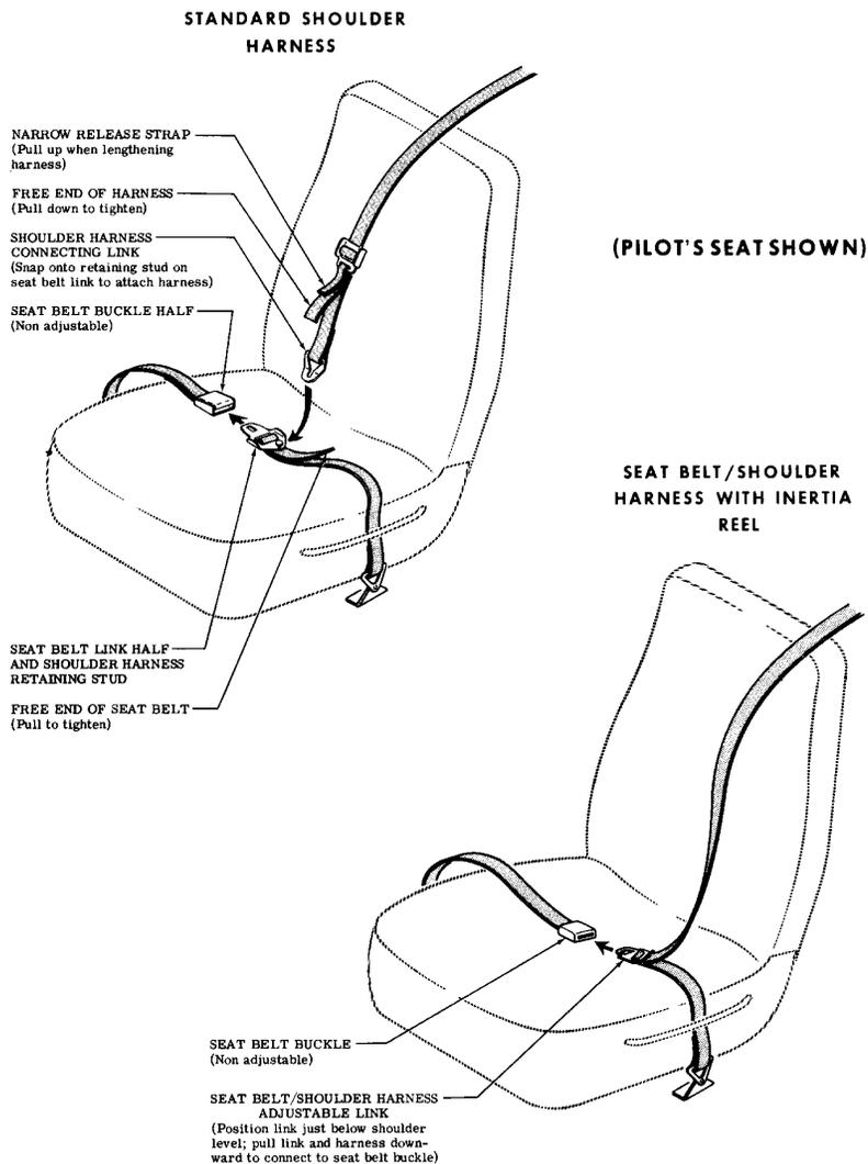
**Figure 7-4. Seat Belts and Shoulder Harnesses**
